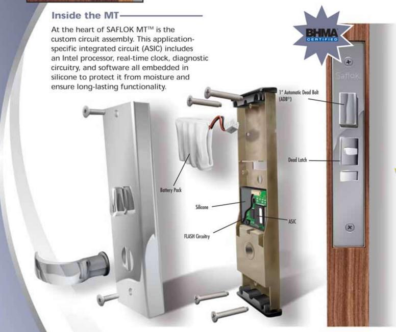
The non-volatile FLASH circuitry stores over a year's worth of lock data (or up to 5,900 entries) providing detailed audit-trail information such as date and time of the entry as well as the ID code of the employee or guest using the keycard.
